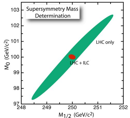
*Together the ILC and LHC can measure the unified supersymmetry masses much more precisely than either machine alone.*
