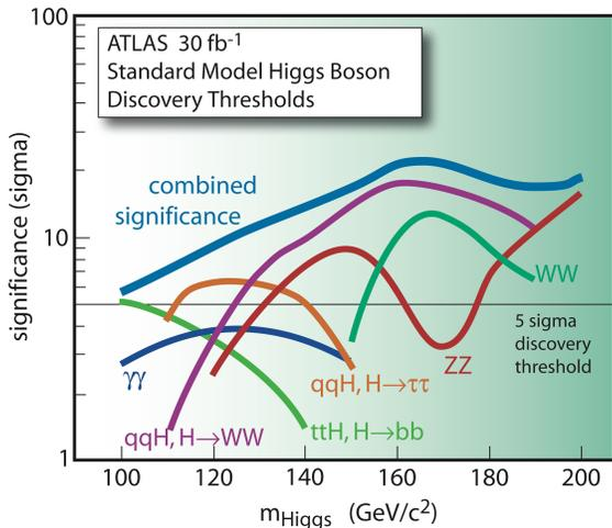
*The LHC can discover a light Standard Model Higgs boson in the initial period of operation in a number of modes.*
