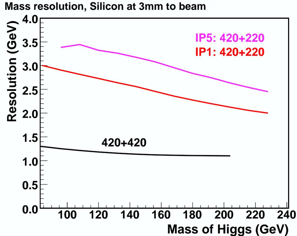
Calculated for silicon 3mm from beam; results similar (given acceptance) for other distances.
